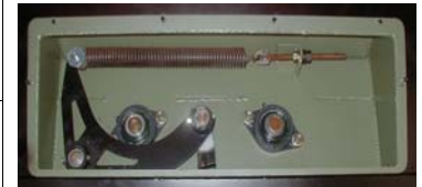
Chain Tensioning Unit
