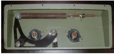
Chain Tensioning Unit
